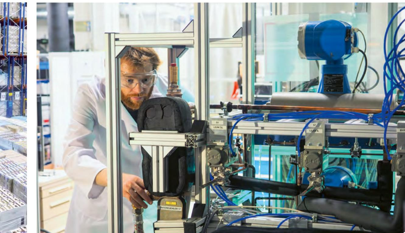
Clemens Dankwerth from Fraunhofer ISE examines a propane refrigeration circuit for leaks in the test laboratory. The refrigeration circuit is one of the central components of the newly developed LC 150 heat pump, which works with propane as its environmentally friendly refrigerant. © Fraunhofer ISE / Marek Miara
