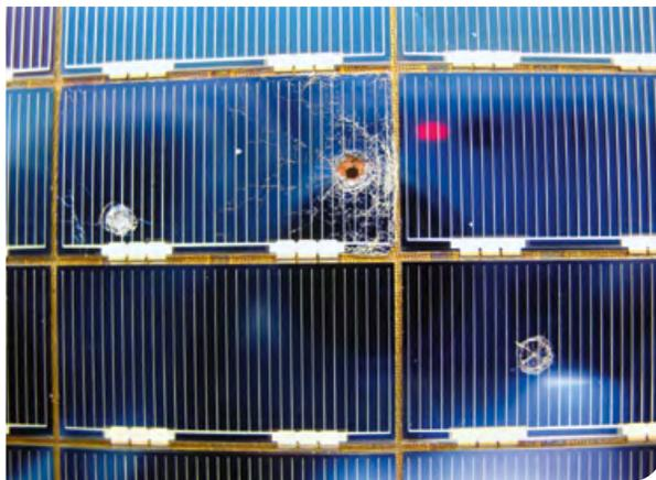
Damage to the Hubble space telescope, which was launched into orbit in 1990. © ESA
