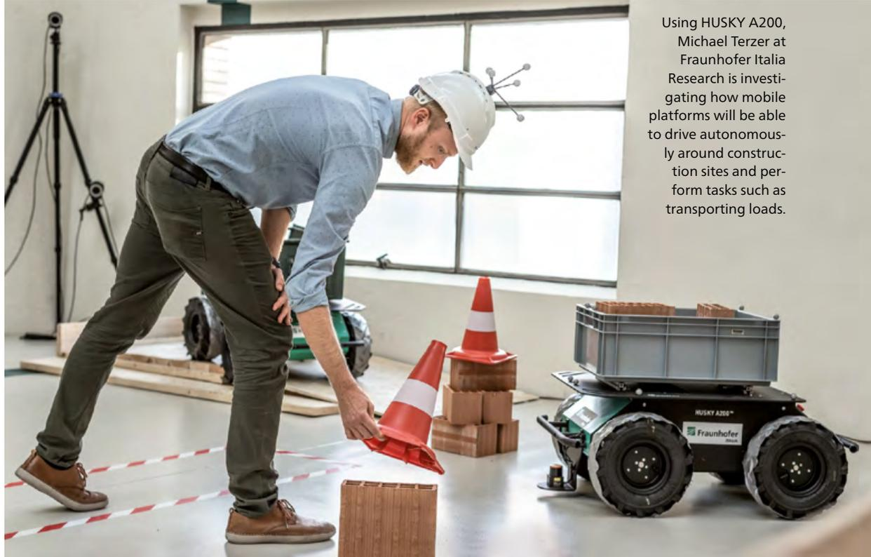
Using HUSKY A200, Michael Terzer at Fraunhofer Italia Research is investigating how mobile platforms will be able to drive autonomously around construction sites and perform tasks such as transporting loads.
